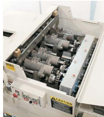
An additional center feed roll can be added for ripping short length stock. The center roll uses a removable sleeve to mount spur drive discs, wooden rolls (shown above) or urethane feed tires. This option accommodates ripping stock as short as 8" long.
